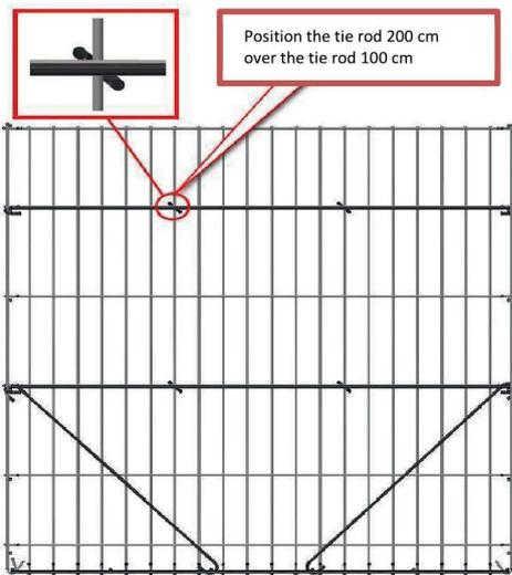
Figure A.13 – Step 11: insert the remaining tie rods, positioning the tie rods of L cm 200 over the tie rods of L cm 100
