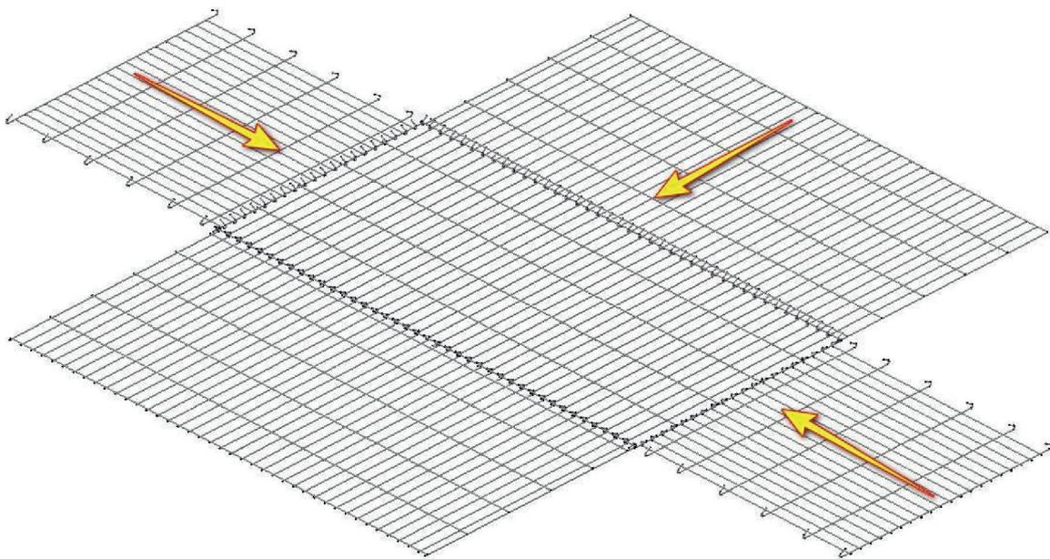
**Figure A.4 – Step 2: connect one plain side panel with bottom panel**
