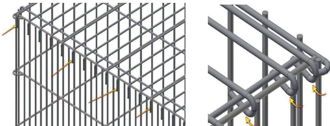
Figure A.15 – Step 13: bend inwards all the 90° laid hooks of the top panel
