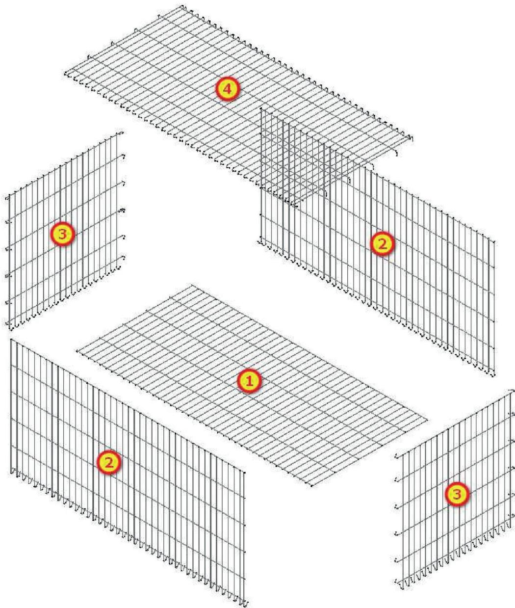
**Figure A.1 – The mesh panels which make up the gabion box**
