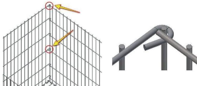
**Figure A.9 – Step 7: by using the pliers close two hooks, the first and the fourth hook of each side panel**
