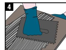
Spread the adhesive for sintered stone on the back of the slabs.
