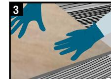
Slabs must adhere to the adhesive layer.
