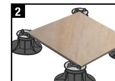
Place the supports in relation to the dimensions of the used tile.
